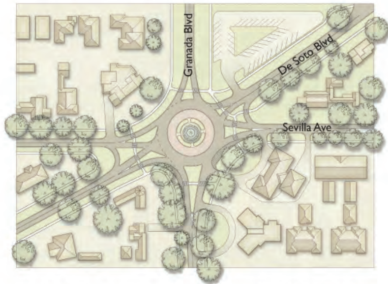
Option 1: Six-Point Roundabout - Leave all streets as they are, resulting in no curb changes and many complex splitter islands.
