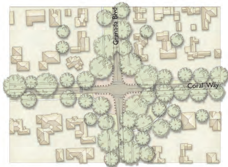
Option 1: Convert to a typical 4-way intersection and create a plaza at each quadrant. The plazas may be flush with the street or have a small curb and they may be separated from the road with bollards, pots, or planters.
