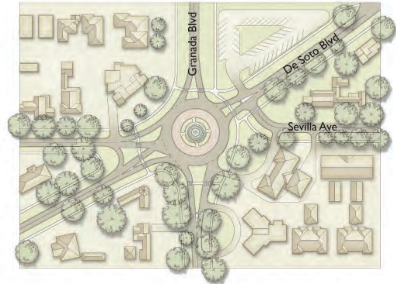
Option 2: Five-Point Roundabout - Merge De Soto Boulevard and Sevilla Avenue at the northeast end, resulting in some curb changes and less splitter islands.
